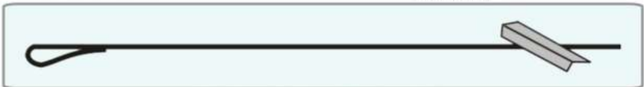
Wire Rope Stay Rod (Size 14mm x 2mtr)
